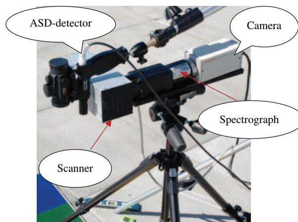
Fig. 1. The components of visible/near-infrared imaging spectrometer.
