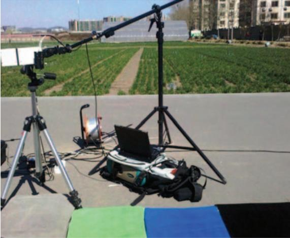
Fig. 6. Reference objects of field calibration.
