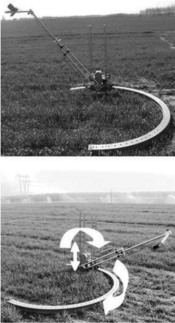
Fig. 1. Rotating bracket for observing BRDF canopy reflectance.
