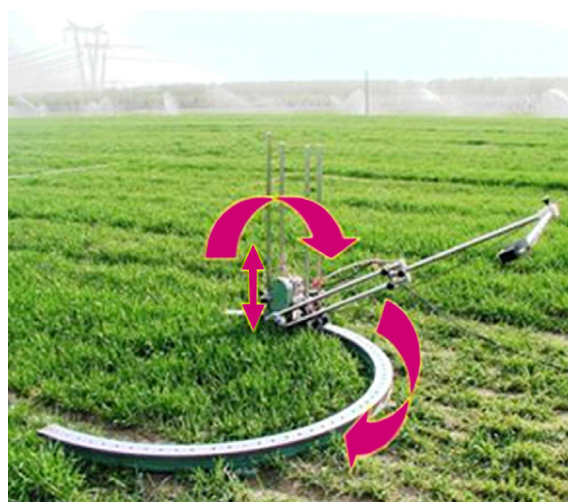
Fig. 1. The rotating bracket for canopy multi-angle spectral measurement. The semi-circular track controls the observation azimuth angle, the rotating boom controls the zenith angles, and the up-and-down arrow indicates that the observation height can be changed according to crop height.
