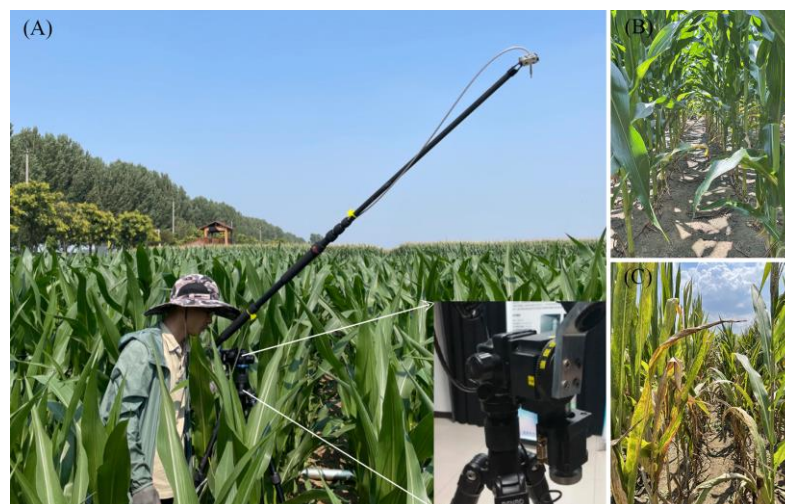
Figure 2. In situ multiangle hyperspectral measurements of maize. (A) is a multiangle hyperspectral measurement device; (B) depicts the early-stage symptoms occurring beneath the canopy of maize plants; (C) illustrates the late stage of the disease, with symptoms covering the entire maize plant.
